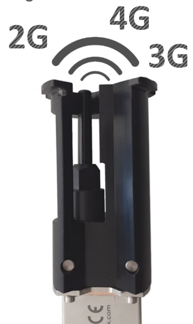
Antenna detachable for connection of an external antenna
